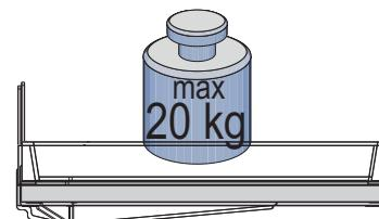
$$+ \text{ (3 weights)} = \Sigma = \text{max } 120 \text{ kg}$$
